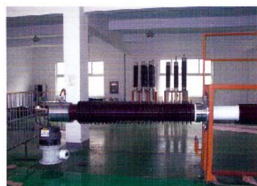
252kV套管极限抗弯实验 Limit cantilever withstand strength test
