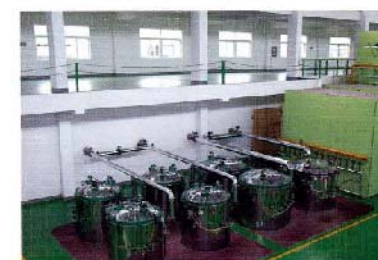
电容芯子真空干燥罐 Vacuum dry can for capacitive core
